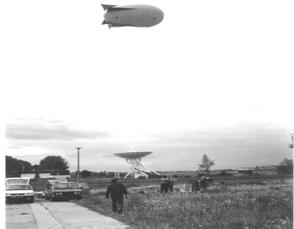
Fig. 4. Transmitter with linear antenna which has been extended to a height of 333-m using a balloon
