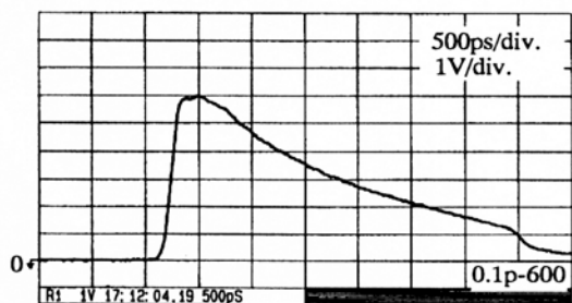
(a) source voltage is 600V
